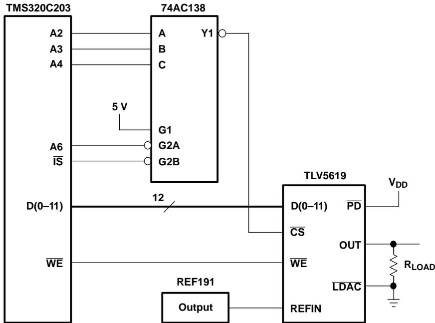
**Figure 13. TLV5619 to TMS320C203 DSP Interface Connection**
