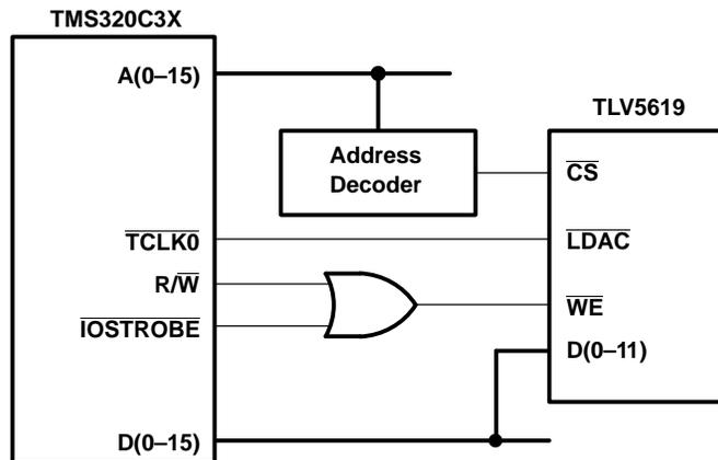
Figure 12. Proposed Interface Between TLV5619 and TMS320C3X DSPs
